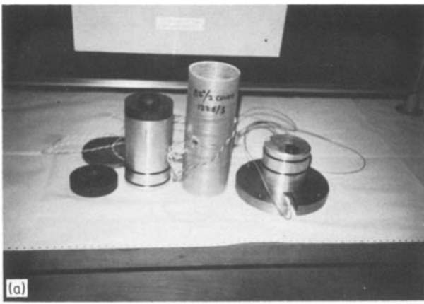
Figure 3 (a, b) A test specimen with its end-plugs. (1) Test specimen, (2) top plug, (3) bottom plug, (4) male top plate, (5) female top plate, (6) lead plate.
